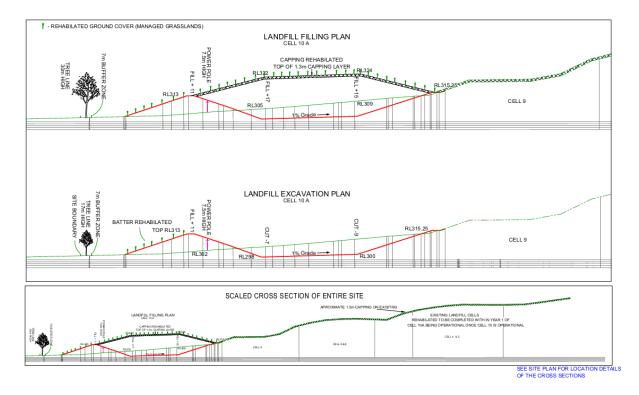
It is considered that the cross section plans overall show more detail than required by the SRPP and facilitate an assessment of visual impact associated with the landfill extension. To further assist in this regard the applicant has provided some modelled video images taken. The link to these have been separately provided to the Panel.
